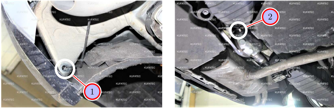
Figure 9: Cable routing to the sound generator
